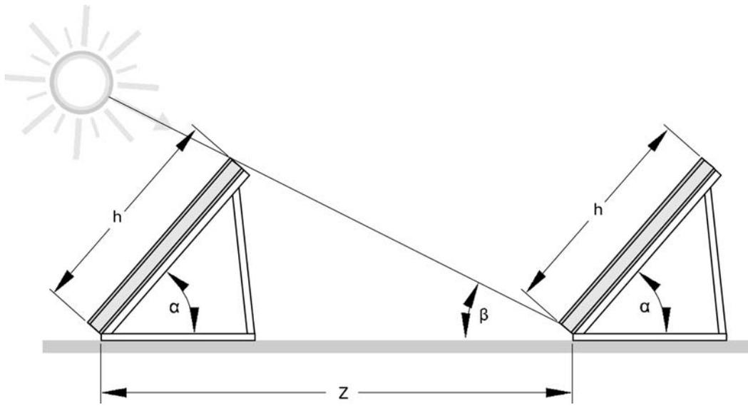
**Determining the collector row clearance z**
