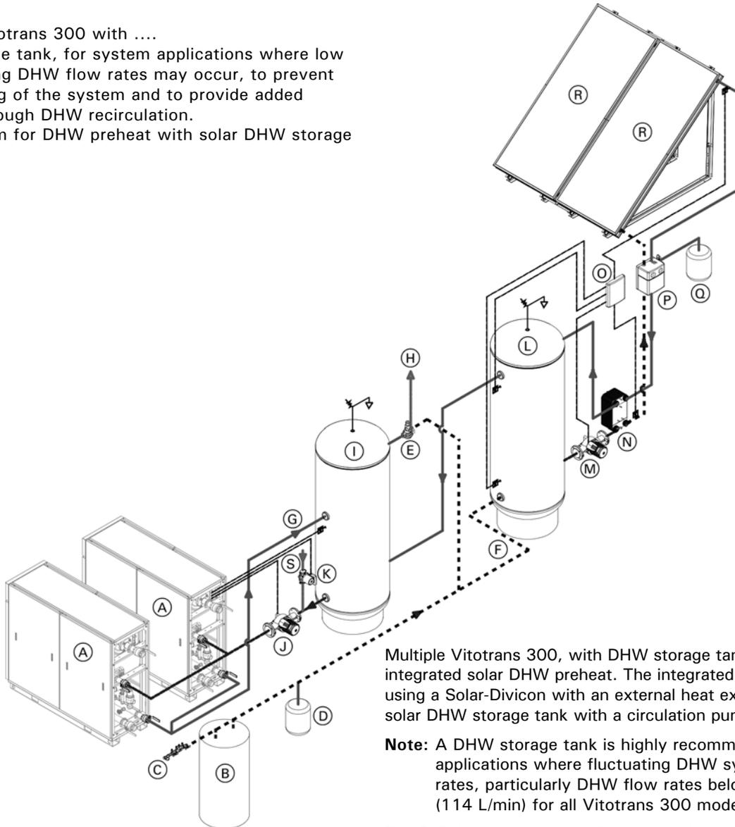
Multiple Vitotrans 300, with DHW storage tank and integrated solar DHW preheat. The integrated solar includes using a Solar-Divicon with an external heat exchanger and solar DHW storage tank with a circulation pump.
