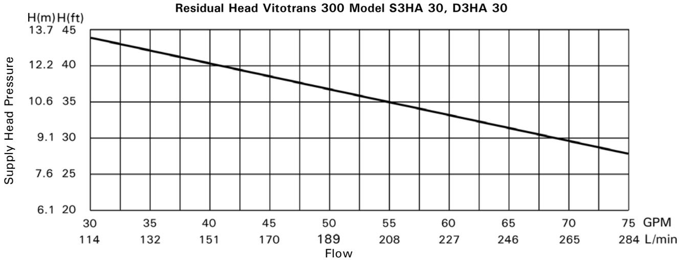
**Note:** Max. system flow 75 GPM (284 L/min)
