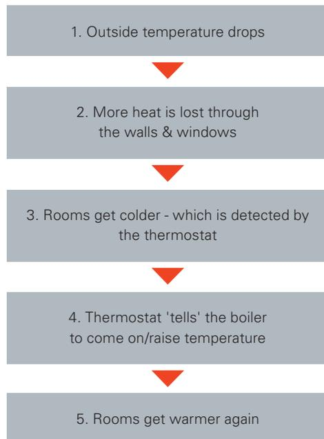
In the previous example, it isn't until stage 4 that the boiler gets any 'feedback' and is able to respond to changing conditions. The chances are that at this stage, the householder will be feeling cold and will turn the thermostat up manually, consuming additional energy.
