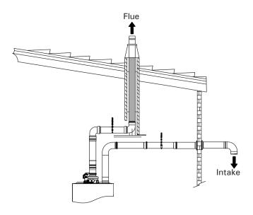
Flexible two pipe system (room air independent)
