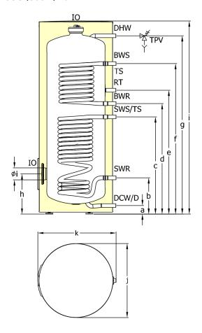
DHW tank temperature sensor in solar heating applications 79 USG (300 L).
