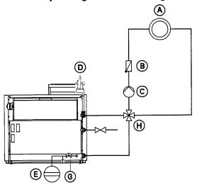
Single-stage operation can only occur when boiler water temperature is above the minimum temperature, and a demand for heat is present. When water temperature is above the minimum, boiler control will determine full input operation or partial load operation based on demand for heat. Refer to boiler control instructions.
