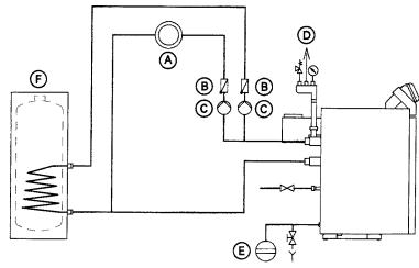
Installation of a spring-loaded flow-check valve in the heating circuit supply as a mechanical "break" is recommended to prevent hot water from flowing unintentionally to (space) heating circuits during priority DHW production or during summer operation (when only DHW is produced).
