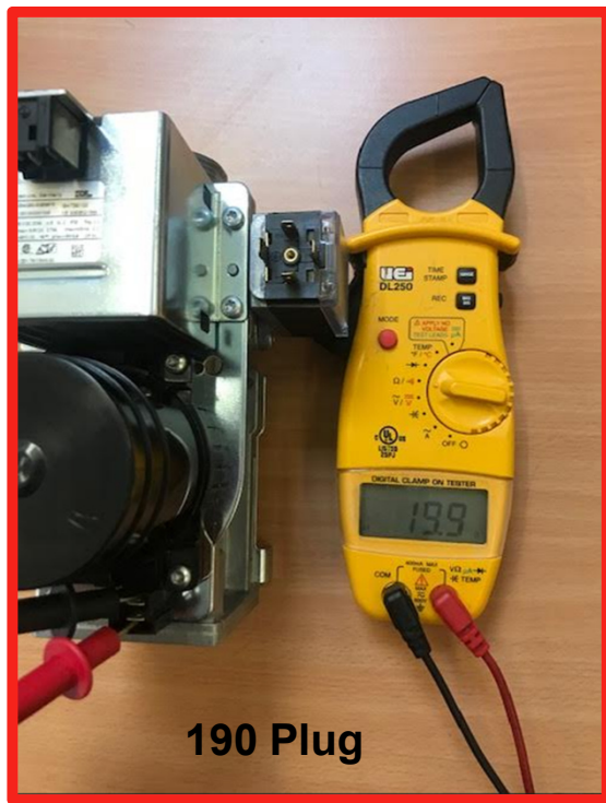
Large Gas Valve 20 ohm
