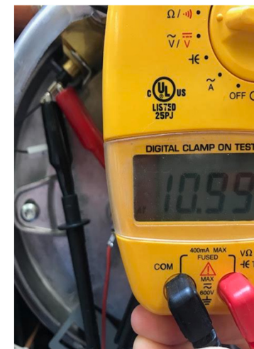
Measure Ohms to check Sensor Accuracy/Drifting
