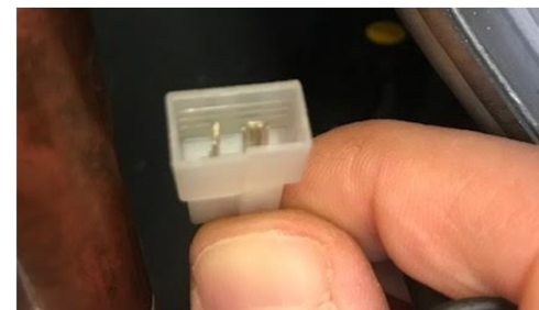
Check continuity of flow switch for proper
