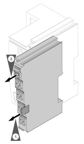
If the gateway or power supply unit need to be removed, e.g. because the device is faulty, proceed as shown in the following diagrams.
