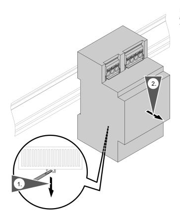
If the gateway or power supply unit need to be removed, e.g. because the device is faulty, proceed as shown in the following diagrams.
