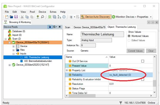
Figure 20: Example – Reliability Property in the WAGO BACnet Configurator
