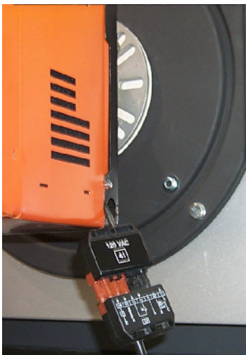
Fig. 13 The quick-connect plug-in system
