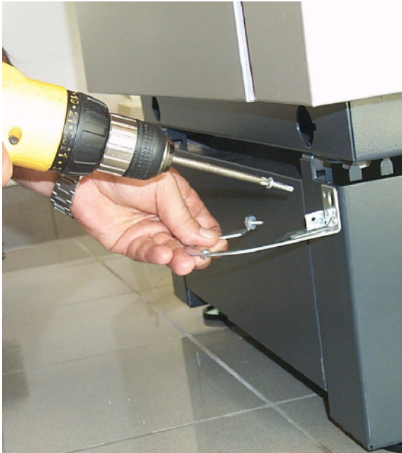
Fig. 7 Side-mounting support bracket
